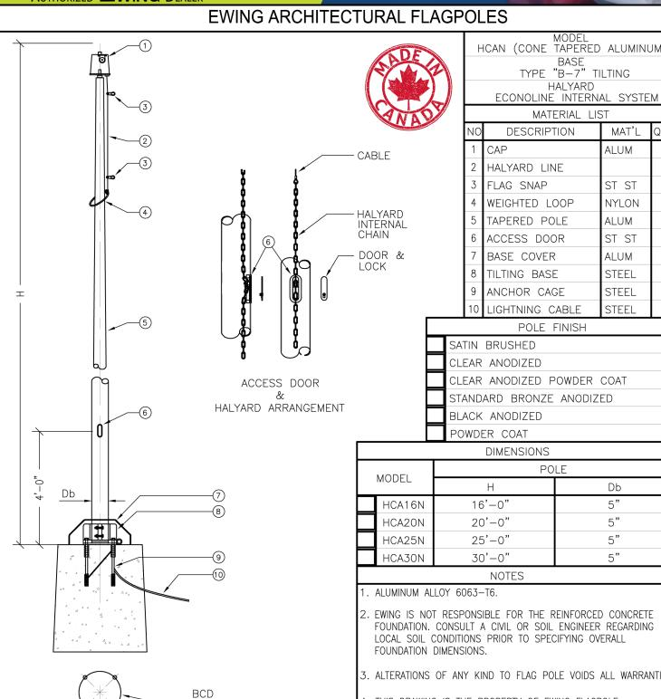
MODEL HCAN (CONE TAPERED ALUMINUM) BASE TYPE "B-7" TILTING HALYARD
